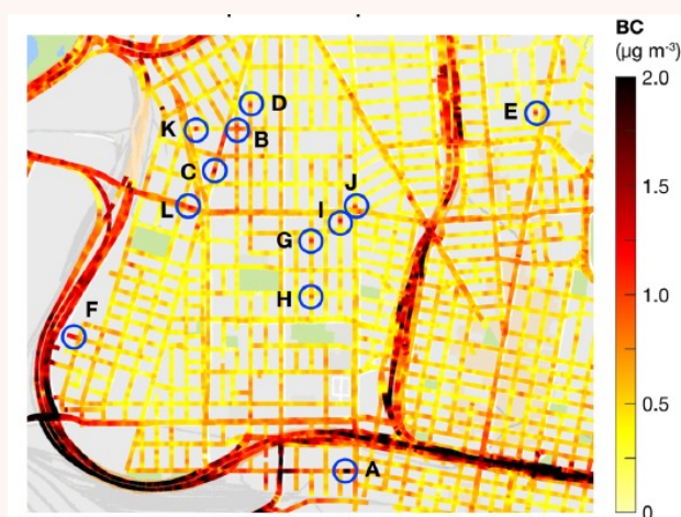
Multipollutant hotspots identified from BC median concentrations measured using the Google Street View cars in Oakland, California.
